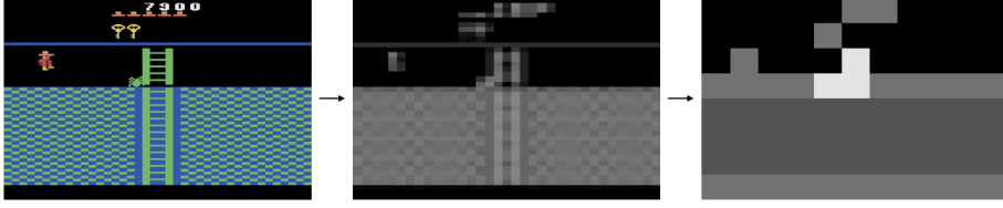
Figure 3.3: An example of cell representation in Go-Explore. The image is first converted to grayscale, then sub-sampled to an 11 \times 8 image containing 8 distinct levels of pixel intensity. The resulting image is the cell representation. Figure from [70].
